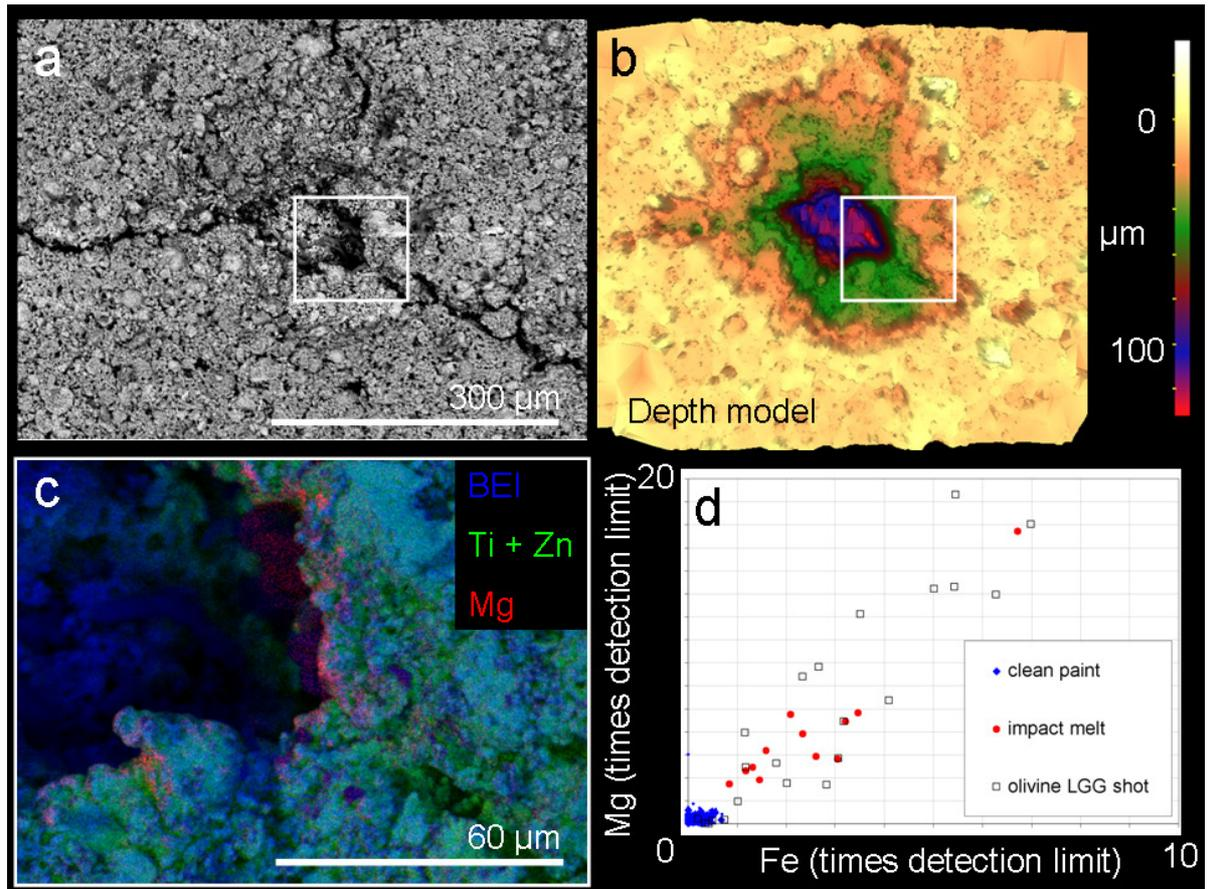
Figure 1. WFPC2 impact 339: a) SEM backscattered electron (BE) image; b) depth model; c) SEM-EDX maps show Mg in impact melt lining the impact feature d) plots of SEM-EDX X-ray counts for Mg and Fe show much higher levels in impact melt (red) than in clean ZOT paint (blue), and similar to impact residue from LGG impacts of olivine grains (open black squares). Excess Mg and Fe in frothy impact melt show impactor was a micrometeoroid.
